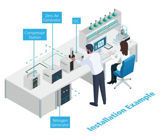
Zero Air Generators provide a clean and stable source of hydrocarbon-free air for the supply of oxidant gas to detectors used in Gas Chromatography systems including:
